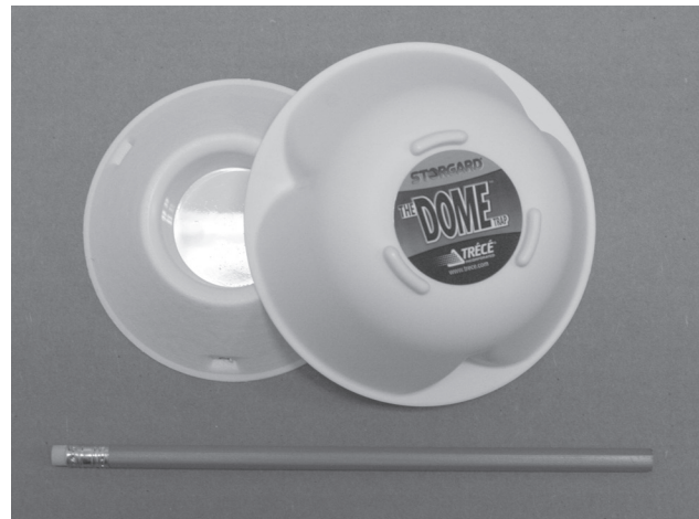
Figure 3. A pitfall trap, a type of specialized surface trap for capturing stored-product beetles.
