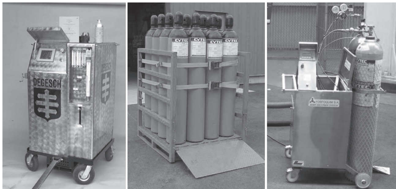
Figure 4. A phosphine generator (left). Cylinder-based phosphine at 2% in carbon dioxide (center) and 100% \text{PH}_3 being diluted immediately in air (right).
