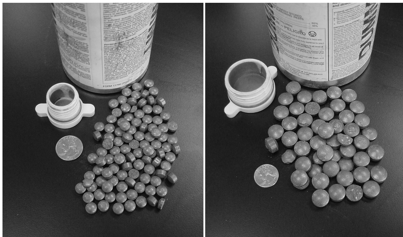
Figure 3. Pellets (left) and tablets (right) of aluminum phosphide that generate 0.2 and 1.0 g, respectively, of phosphine each when fully reacted.
