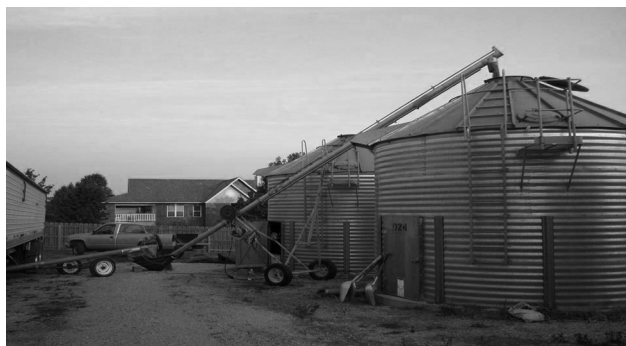
Figure 2. Wheat being loaded into a small-scale bin. The protectant insecticide is often applied as the grain is falling into the auger boot (photo courtesy of F. H. Arthur, USDA-ARS-CGAHR).
